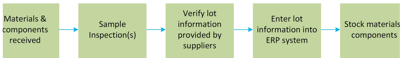
Pasternack's incoming material flow process
