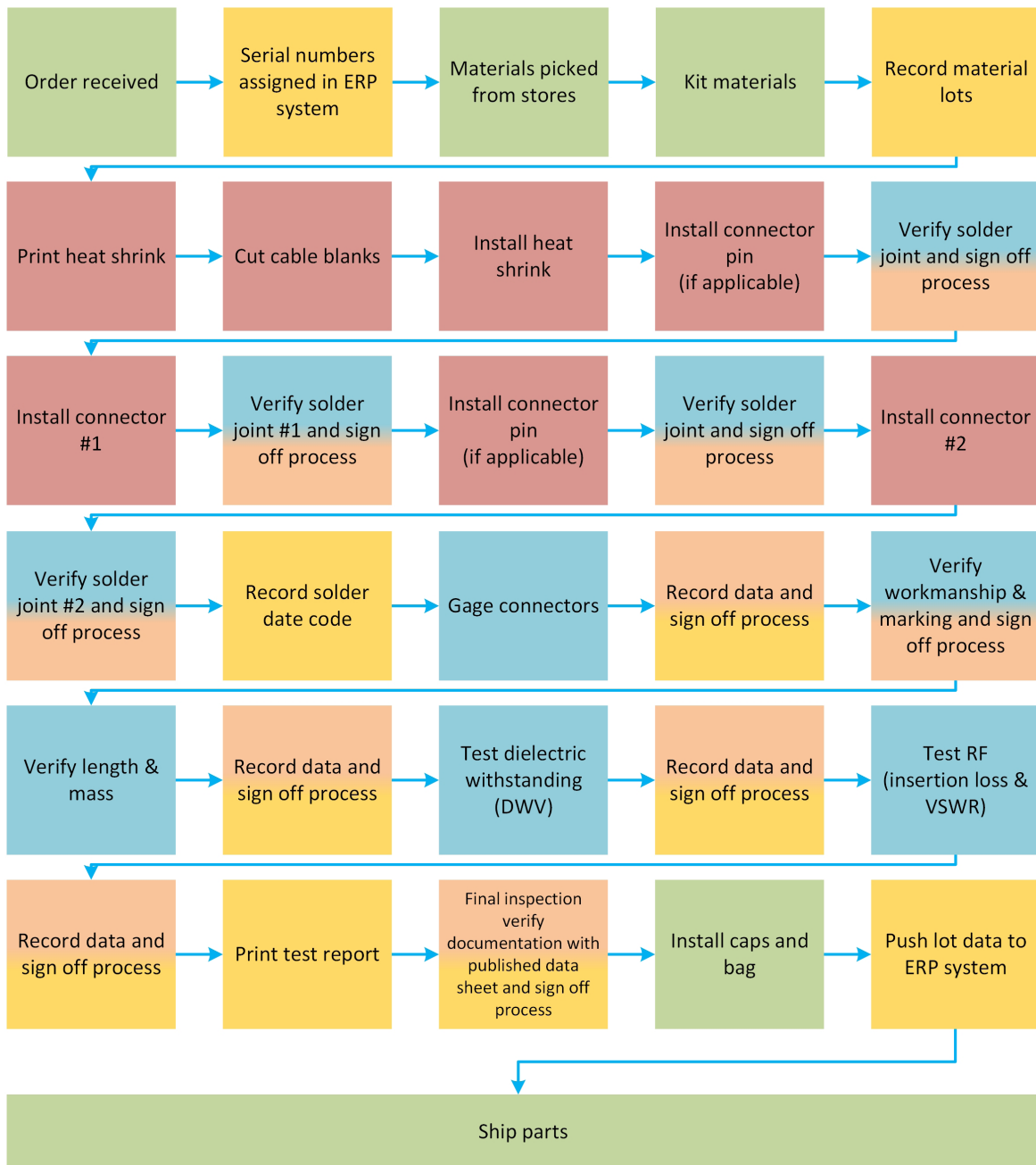
Pasternack's Order Processing Flow for Coaxial Cable Assemblies
