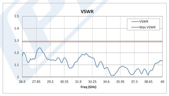
Click the following link (or enter part number in "SEARCH" on website) to obtain additional part information including price, inventory and certifications: WR-28 UG-599/U Square Cover Flange to 2.92mm Male Waveguide to Coax Adapter Operating from 26.5 GHz to 40 GHz PE-W28CA002
