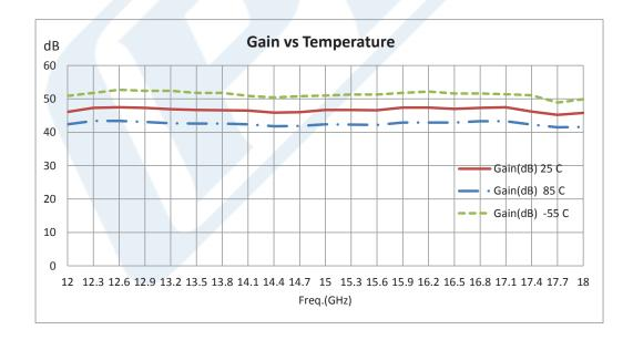
Click the following link (or enter part number in "SEARCH" on website) to obtain additional part information including price, inventory and certifications: 43 dB Gain, 1 Watt, 12 GHz to 18 GHz, Broadband High Gain Amplifier, 39 dBm IP3, 6 dB NF, SMA PE15A3507
