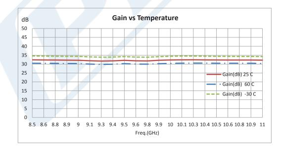
Click the following link (or enter part number in "SEARCH" on website) to obtain additional part information including price, inventory and certifications: 1 Watt P1dB, 8.5 GHz to 11 GHz, Medium Power GaAs Amplifier, SMA Input, SMA Output, 30 dB Gain, 38 dBm IP3, 3 dB NF PE15A4006
