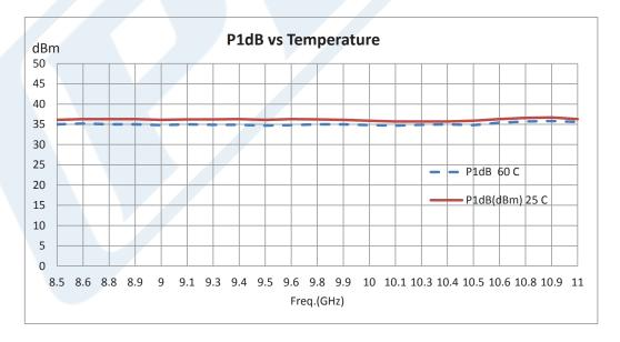
Click the following link (or enter part number in "SEARCH" on website) to obtain additional part information including price, inventory and certifications: 4 Watt P1dB, 8.5 GHz to 11 GHz, High Power GaAs Amplifier, SMA Input, SMA Output, 30 dB Gain, 45 dBm IP3, 5 dB NF PE15A4007
