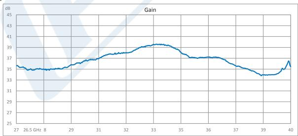
Click the following link (or enter part number in "SEARCH" on website) to obtain additional part information including price, inventory and certifications: 22 dBm Psat, 26.5 GHz to 40 GHz, Medium Power Amplifier, 2.92mm Input, 2.92mm Output, 35 dB Gain, 28 dBm IP3, 4.5 dB NF PE15A4050
