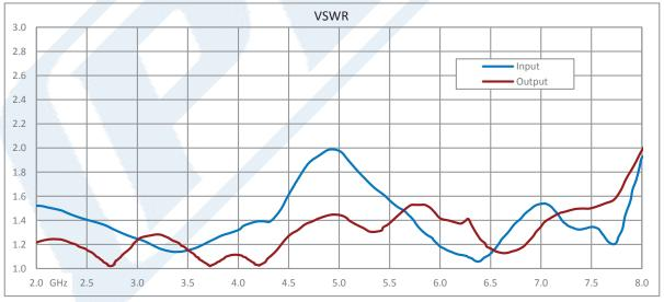
Click the following link (or enter part number in "SEARCH" on website) to obtain additional part information including price, inventory and certifications: 1 Watt P1dB, 2 GHz to 8 GHz, Medium Power Amplifier, SMA, 38 dB Gain, 5.5 dB NF PE15A4054
