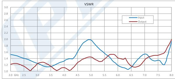
Click the following link (or enter part number in "SEARCH" on website) to obtain additional part information including price, inventory and certifications: 1 Watt P1dB, 2 GHz to 8 GHz, Medium Power Amplifier with Heatsink, SMA, 38 dB Gain, 5.5 dB NF PE15A4054F
