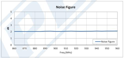
Click the following link (or enter part number in "SEARCH" on website) to obtain additional part information including price, inventory and certifications: 42 dB Gain, 18 Watt Psat, 860 MHz to 960 MHz, High Power Amplifier, SMA Input, SMA Output, 55 dBm IP3, 3.5 dB NF PE15A5042
