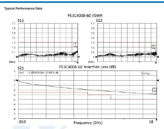
Click the following link (or enter part number in "SEARCH" on website) to obtain additional part information including price, inventory and certifications: Handheld RF Analyzer Rugged Phase Stable Cable N Male to SMA Male Cable 60 Inch Length Using PE-FF430 Coax, RoHS PE3C4008-60
