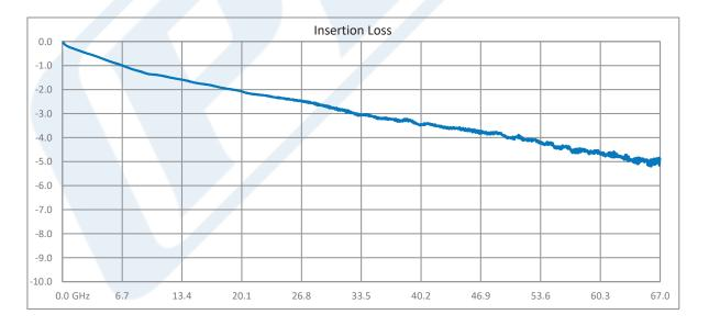
Measurement is for two connectors with 1.0 inch (25.4mm) length of substrate
