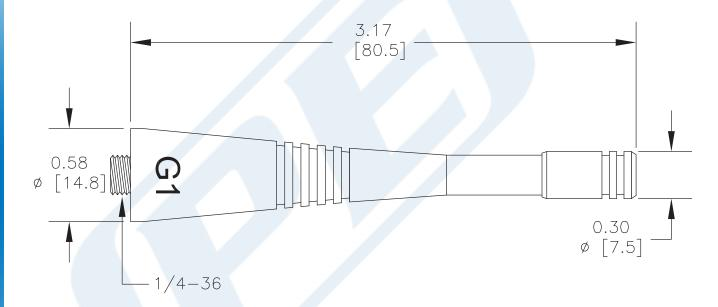
Click the following link (or enter part number in "SEARCH" on website) to obtain additional part information including price, inventory and certifications: Whip Antenna Operates From 806 MHz to 880 MHz With a Typical 0 dBi Gain SMA Female Input Connector IP67 Rated PE51156
