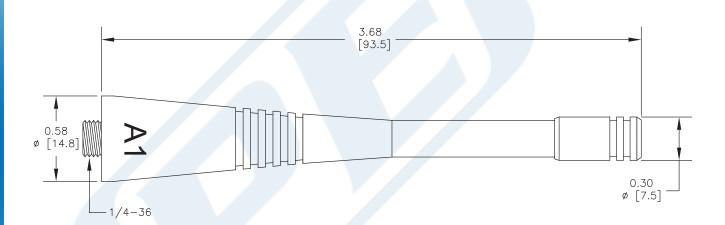
Click the following link (or enter part number in "SEARCH" on website) to obtain additional part information including price, inventory and certifications: Whip Antenna Operates From 698 MHz to 780 MHz With a Typical 0 dBi Gain SMA Female Input Connector IP67 Rated PE51157
