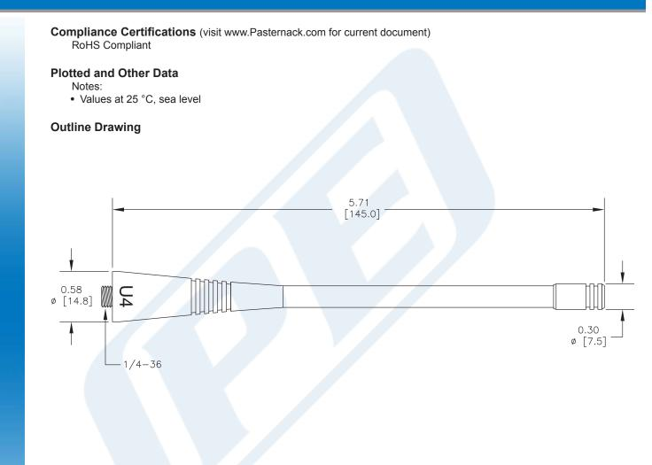
Click the following link (or enter part number in "SEARCH" on website) to obtain additional part information including price, inventory and certifications: Whip Antenna Operates From 470 MHz to 512 MHz With a Typical 0 dBi Gain SMA Female Input Connector IP67 Rated PE51161
