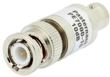
10 dB Fixed Attenuator, BNC Male to BNC Female Brass Nickel Body Rated to 1 Watt Up to 2 GHz from Pasternack Enterprises has same day shipment for domestic and International orders. Our RF, microwave and millimeter wave products maintain a 99.4% availability and are part of the broadest selection in the industry.
