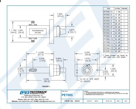
0 to 7 dB Rotary Continuously Variable Attenuator, SMA Female To SMA Female Rated To 5 Watts From 1000 MHz To 2 GHz from Pasternack Enterprises has same day shipment for domestic and International orders. Our RF, microwave and millimeter wave products maintain a 99% availability and are part of the broadest selection in the industry.
