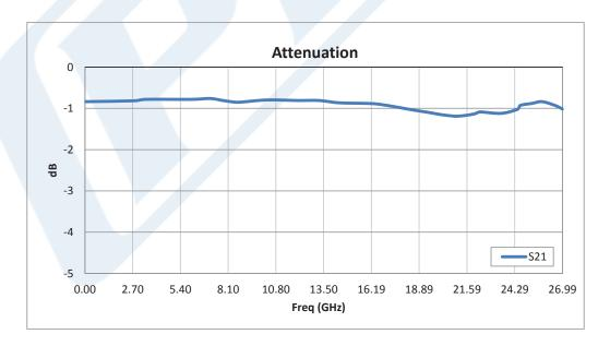
Click the following link (or enter part number in "SEARCH" on website) to obtain additional part information including price, inventory and certifications: 1 dB Fixed Attenuator, SMA Male to SMA Female Passivated Stainless Steel Body Rated to 2 Watts Up to 26 GHz PE7087-1
