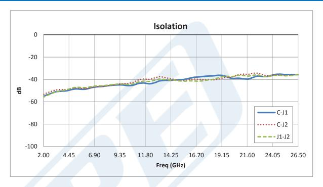
SPDT PIN Diode Switch Operating From 2 GHz to 26.5 GHz Up to +30 dBm and SMA from Pasternack Enterprises has same day shipment for domestic and International orders. Our RF, microwave and millimeter wave products maintain a 99.4% availability and are part of the broadest selection in the industry.
