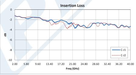
Click the following link (or enter part number in "SEARCH" on website) to obtain additional part information including price, inventory and certifications: SPDT PIN Diode Switch Operating From 2 GHz to 40 GHz Up to +27 dBm and 2.92mm PE71S2021
