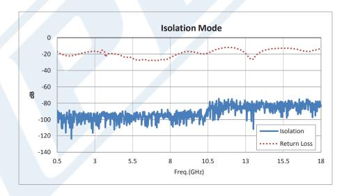
Absorptive SPDT PIN Diode Switch Operating From 500 MHz to 18 GHz Up to +20 dBm and Field Replaceable SMA from Pasternack Enterprises has same day shipment for domestic and International orders. Our RF, microwave and millimeter wave products maintain a 99% availability and are part of the broadest selection in the industry.
