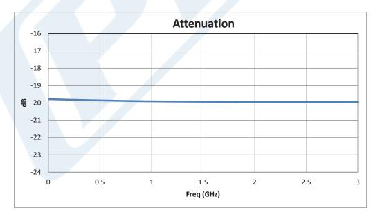
Click the following link (or enter part number in "SEARCH" on website) to obtain additional part information including price, inventory and certifications: 20 dB Fixed Attenuator, N Male to N Female Unidirectional Black Anodized Aluminum Heatsink Body Rated to 50 Watts Up to 3 GHz PE7388-20
