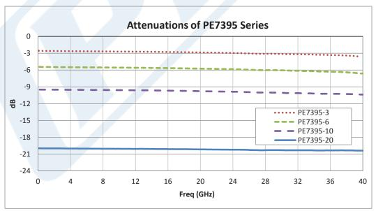
Click the following link (or enter part number in "SEARCH" on website) to obtain additional part information including price, inventory and certifications: 15 dB Fixed Attenuator, 2.92mm Male to 2.92mm Female Passivated Stainless Steel Body Rated to 2 Watts Up to 40 GHz PE7395-15
