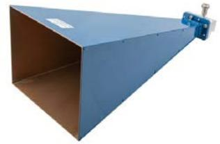
WR-137 Standard Gain Horn Antenna Operating From 5.85 GHz to 8.2 GHz, 20 dBi Nominal Gain, Type N Female Input Connector, ProLine
