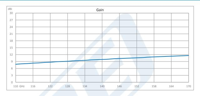
WR-6 Waveguide Standard Gain Horn Antenna Operating from 110 GHz to 170 GHz with a Nominal 10 dBi Gain with UG-387/U-Mod Round Cover Flange from Pasternack Enterprises has same day shipment for domestic and International orders. Our RF, microwave and millimeter wave products maintain a 99.4% availability and are part of the broadest selection in the industry.
