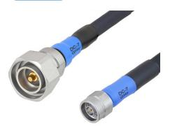
Pasternack's line of test cables for handheld RF analyzers consists of 19 models designed to deliver optimal amplitude and phase stability with flexure. The portable radio frequency analyzer cable series boasts VSWR as low as 1.2:1 and maximum operating frequency of 27 GHz, depending on the configuration. These rugged RF handheld portable analyzer test cables feature crush resistance of 1200 psi and operating temperature range of -55°C to +105°C.
