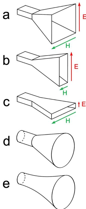
(a) a pyramidal gain horn shaped as a four-sided pyramid with a rectangular cross section aperture and constant flare angle (b) a E-plane rectangular horn antenna (c) a H-plane rectangular horn antenna (d) a conical horn antenna with a circular aperture and a constant flare angle (e) a conical horn antenna with an exponential flare angle.
