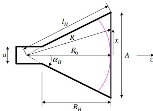
The electrical length of a gain horn antenna is a function of frequency. Hence, higher frequency signals experience a larger electrical length for the same size antenna as lower frequency signals. This is why gain and directivity of a gain horn increases as a function of frequency and beamwidth decreases.
