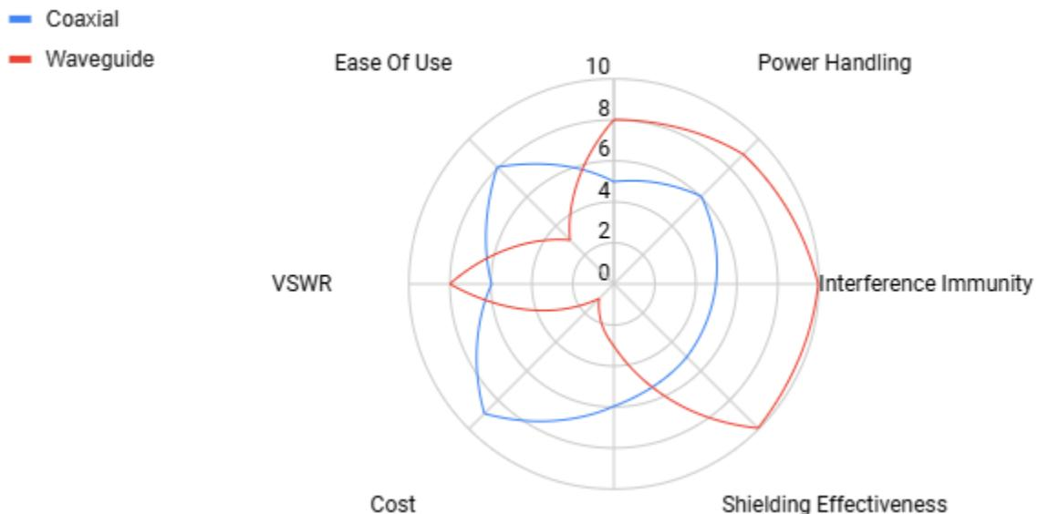
Image: A chart depicting the relative comparison of coaxial transmission lines and waveguides for RF applications.
