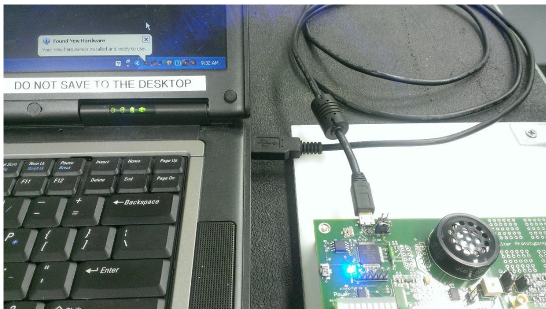
Figure 3: PEM11002-KIT Connected to Laptop Using a USB Cable
