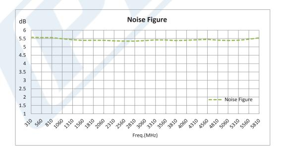
Click the following link (or enter part number in "SEARCH" on website) to obtain additional part information including price, inventory and certifications: 29 dBm P1dB, 60 MHz to 6 GHz, Medium Power GaAs Amplifier, SMA Input, SMA Output, 36 dB Gain, 39 dBm IP3, 5 dB NF PE15A4019
