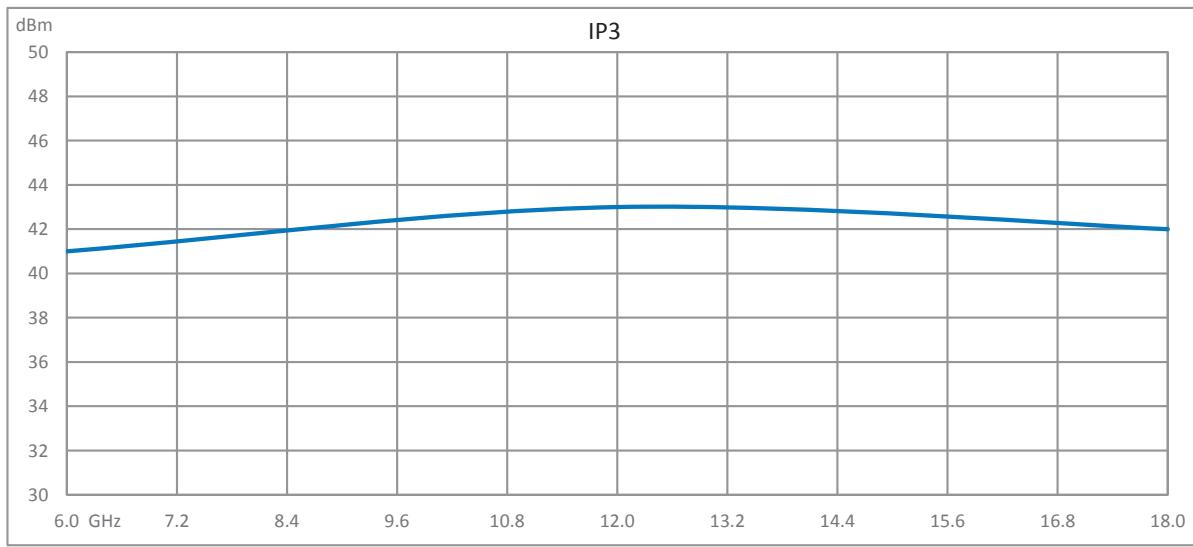
2 Watt P1dB, 6 GHz to 18 GHz, Medium Power Amplifier
