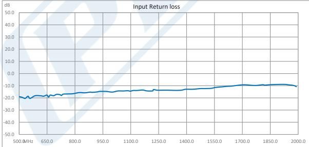
Click the following link (or enter part number in "SEARCH" on website) to obtain additional part information including price, inventory and certifications: 43 dB Gain, 20 Watt Psat, 0.5 GHz to 2 GHz, High Power GaN Amplifier, Class AB, SMA PE15A5111
