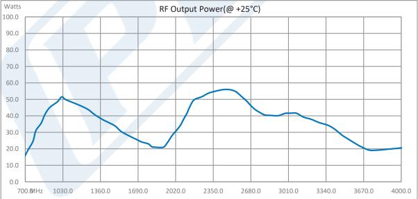
Click the following link (or enter part number in "SEARCH" on website) to obtain additional part information including price, inventory and certifications: 43 dB Gain, 20 Watt Psat, 0.7 GHz to 4 GHz, High Power GaN Amplifier, Class AB, SMA PE15A5117
