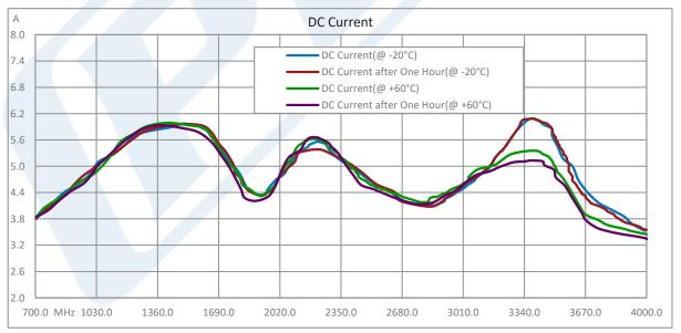
Click the following link (or enter part number in "SEARCH" on website) to obtain additional part information including price, inventory and certifications: 43 dB Gain, 20 Watt Psat, 0.7 GHz to 4 GHz, High Power GaN Amplifier, Class AB, SMA PE15A5117
