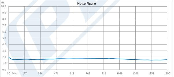
Click the following link (or enter part number in "SEARCH" on website) to obtain additional part information including price, inventory and certifications: 1.6 dB NF Input Protected Low Noise Amplifier, Operating from 30 MHz to 1.5 GHz with 25 dB Gain, 22 dBm P1dB and SMA PE15A63002
