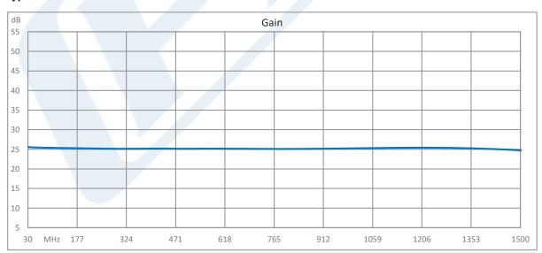
Click the following link (or enter part number in "SEARCH" on website) to obtain additional part information including price, inventory and certifications: 1.6 dB NF Input Protected Low Noise Amplifier, Operating from 30 MHz to 1.5 GHz with 25 dB Gain, 22 dBm P1dB and SMA PE15A63002
