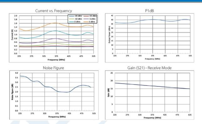
VHF/UHF BiDirectional Amplifier, 225 MHz to 512 MHz 16W Psat, 35% Efficiency, 8 usec Switching, 36dB Tx Gain, Manual T/R Control, SMA from Pasternack Enterprises has same day shipment for domestic and International orders. Our RF, microwave and millimeter wave products maintain a 99.4% availability and are part of the broadest selection in the industry.
