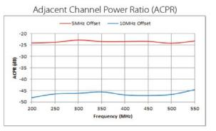
Click the following link (or enter part number in "SEARCH" on website) to obtain additional part information including price, inventory and certifications: VHF/UHF BiDirectional Amplifier, 225 MHz to 512 MHz 16W Psat, 35% Efficiency, 8 usec Switching, 36dB Tx Gain, Manual T/R Control, SMA PE15B5007
