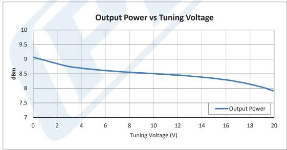
Click the following link (or enter part number in "SEARCH" on website) to obtain additional part information including price, inventory and certifications: Surface Mount (SMT) Voltage Controlled Oscillator (VCO) From 10 MHz to 20 MHz, Phase Noise of -120 dBc/Hz and 0.5 inch Package PE1V11000
