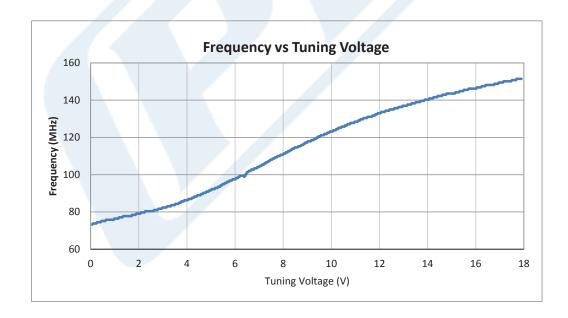
Click the following link (or enter part number in "SEARCH" on website) to obtain additional part information including price, inventory and certifications: Surface Mount (SMT) Voltage Controlled Oscillator (VCO) From 75 MHz to 150 MHz, Phase Noise of -110 dBc/Hz and 0.5 inch Package PE1V11008
