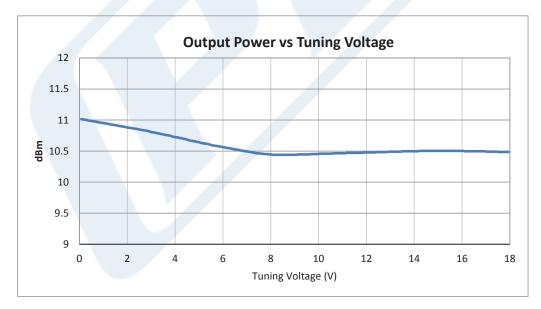
Click the following link (or enter part number in "SEARCH" on website) to obtain additional part information including price, inventory and certifications: Surface Mount (SMT) Voltage Controlled Oscillator (VCO) From 75 MHz to 150 MHz, Phase Noise of -110 dBc/Hz and 0.5 inch Package PE1V11008
