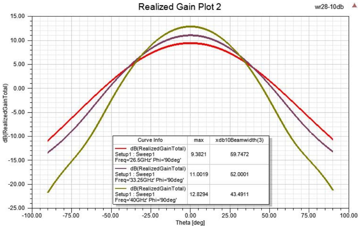
WR-28 Waveguide Antenna, 26.5 GHz to 40 GHz Frequency Range, 10 dBi Gain, UG-599/U Flange, Integrated Cage-Style Mount from Pasternack Enterprises has same day shipment for domestic and International orders. Our RF, microwave and millimeter wave products maintain a 99.4% availability and are part of the broadest selection in the industry.
