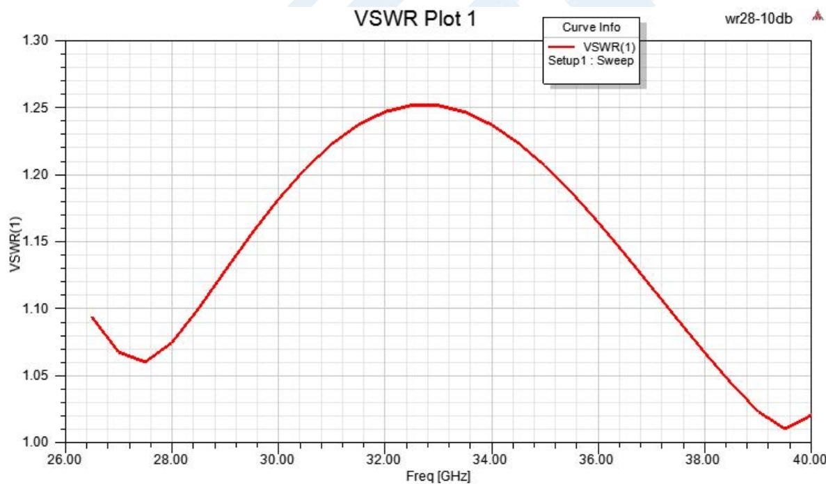
Click the following link (or enter part number in "SEARCH" on website) to obtain additional part information including price, inventory and certifications: [WR-28 Waveguide Antenna, 26.5 GHz to 40 GHz Frequency Range, 10 dBi Gain, UG-599/U Flange, Integrated Cage-Style Mount PE1WAN028-10](#)
