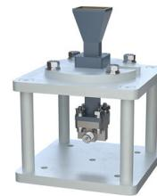
WR-28 Standard Gain Horn with 15 dBi gain, 2.92mm Female connector, Integrated Cage-Style Mount
