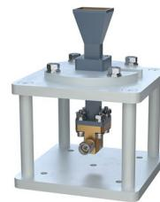
WR-28 Standard Gain Horn with 15 dBi gain, 2.92mm Male connector, Integrated Cage-Style Mount
