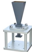
WR-28 Waveguide Antenna, 26.5 GHz to 40 GHz Frequency Range, 20 dBi Gain, UG-599/U Flange, Integrated Cage-Style Mount
