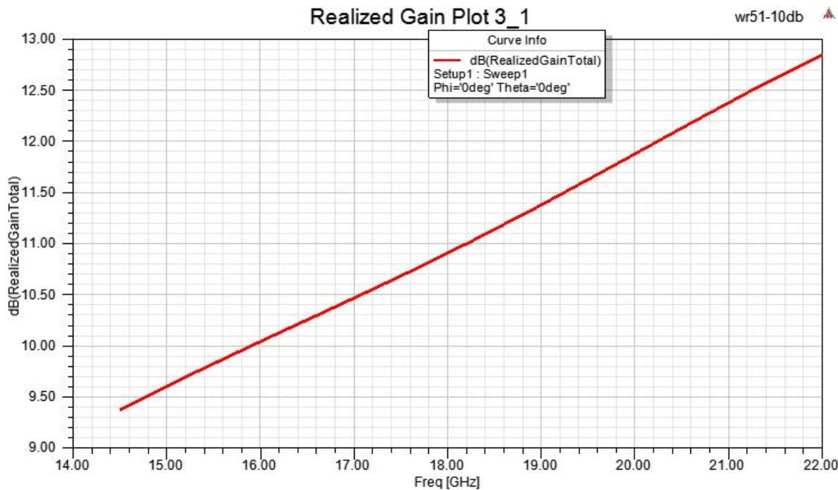
WR-51 Standard Gain Horn with 10 dBi gain, End Launch
