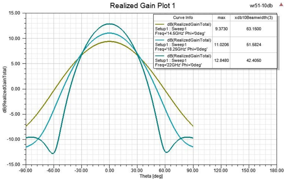
WR-51 Standard Gain Horn with 10 dBi gain, End Launch
