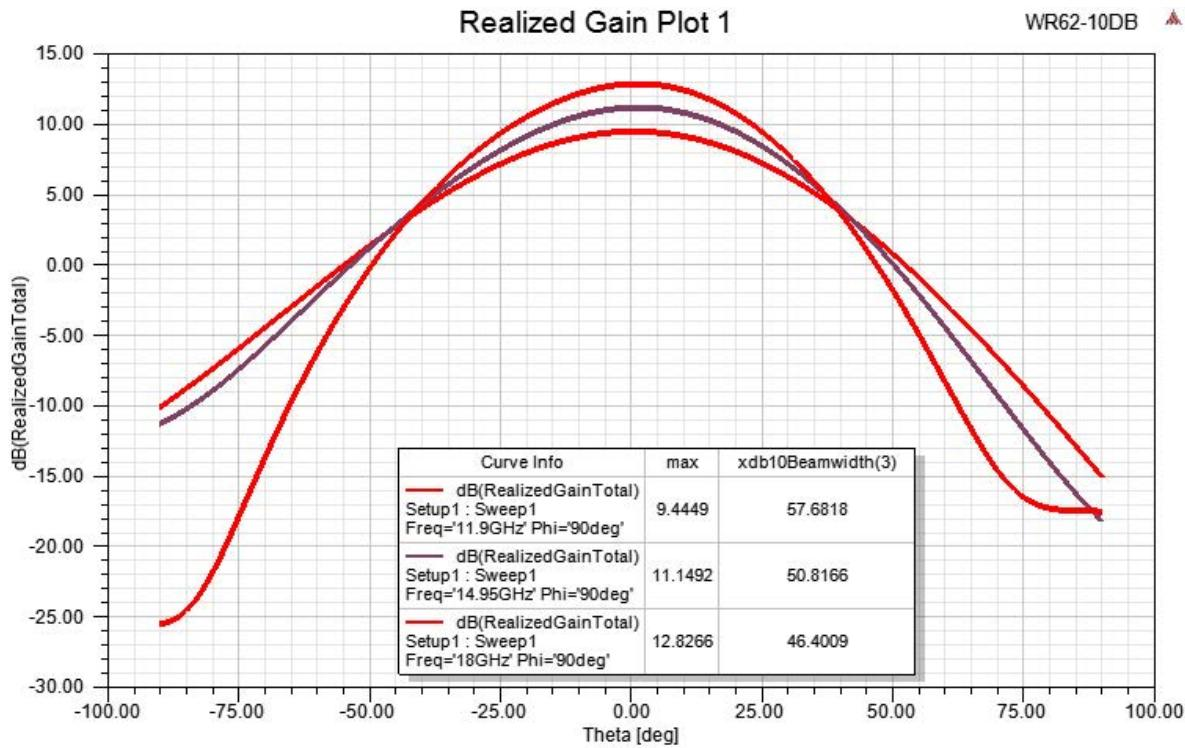
WR-62 Standard Gain Horn with 10 dBi gain, End Launch SMA Female connector, Integrated Cage-Style Mount from Pasternack Enterprises has same day shipment for domestic and International orders. Our RF, microwave and millimeter wave products maintain a 99.4% availability and are part of the broadest selection in the industry.
