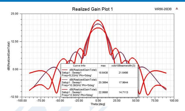
WR-90 Standard Gain Horn with 20 dBi gain, SMA Female connector, Integrated Cage-Style Mount from Pasternack Enterprises has same day shipment for domestic and International orders. Our RF, microwave and millimeter wave products maintain a 99.4% availability and are part of the broadest selection in the industry.
