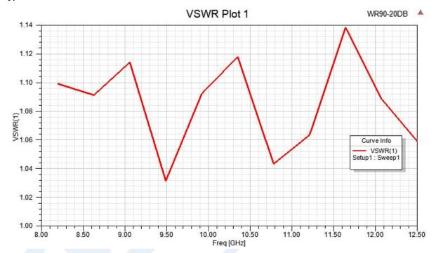
Click the following link (or enter part number in "SEARCH" on website) to obtain additional part information including price, inventory and certifications: WR-90 Standard Gain Horn with 20 dBi gain, SMA Male connector, Integrated Cage-Style Mount PE1WAN090-20SM
