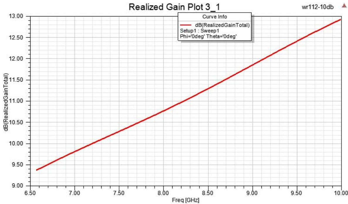
WR-112 Standard Gain Horn with 10 dBi gain, End Launch
