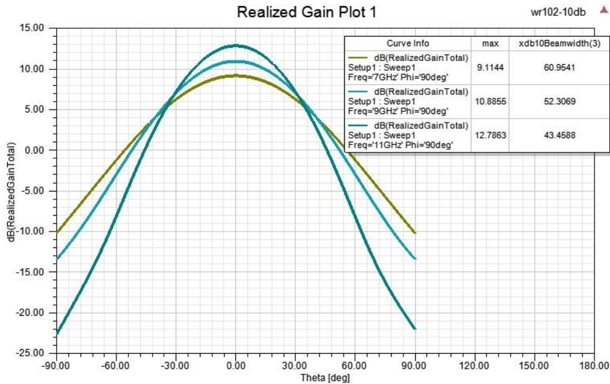
WR-112 Standard Gain Horn with 10 dBi gain, End Launch
