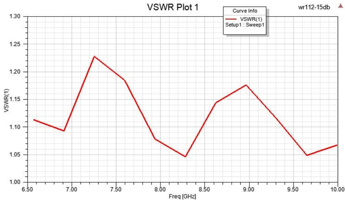
WR-112 Standard Gain Horn with 15 dBi gain, End Launch
