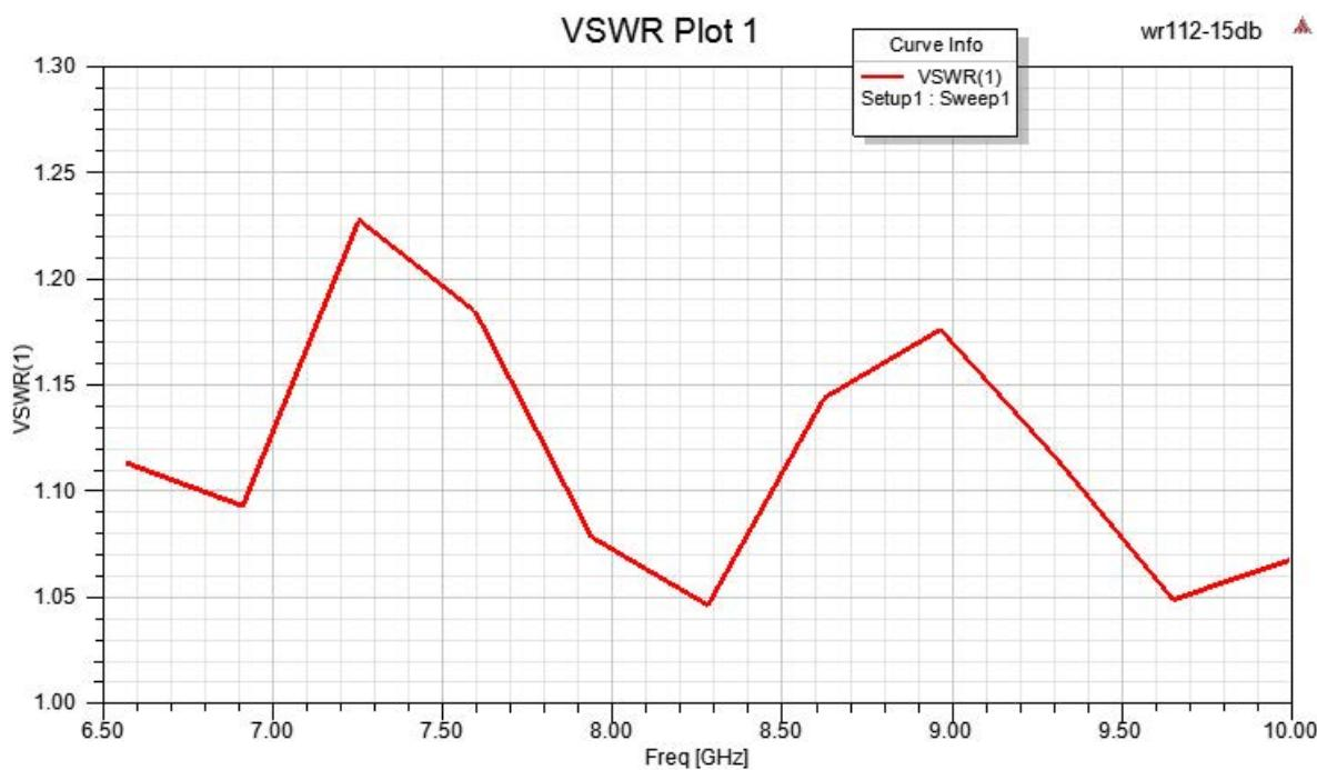
WR-112 Standard Gain Horn with 15 dBi gain, SMA
