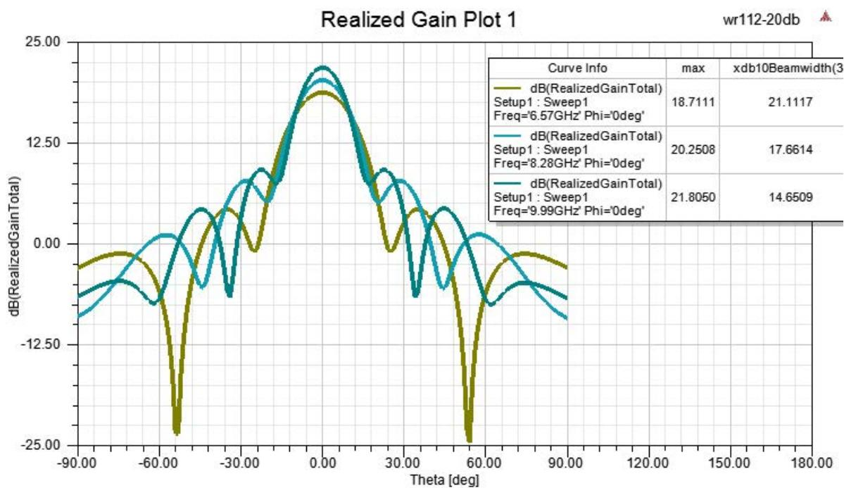
WR-112 Standard Gain Horn with 20 dBi gain, End Launch
