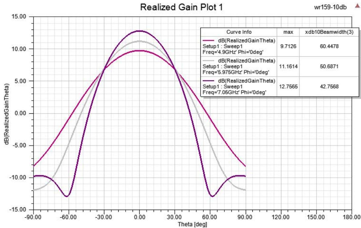
WR-159 Standard Gain Horn with 10 dBi gain, N Female Connector, Integrated Cage-Style Mount
