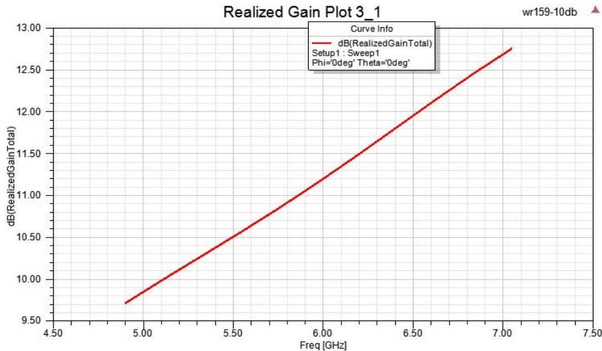
WR-159 Standard Gain Horn with 10 dBi gain, N Female Connector, Integrated Cage-Style Mount
