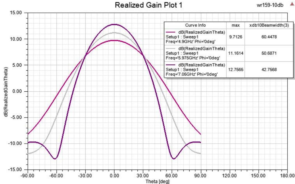
WR-159 Standard Gain Horn with 10 dBi gain, SMA Female Connector, Integrated Cage-Style Mount
