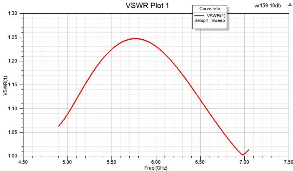
WR-159 Standard Gain Horn with 10 dBi gain, SMA
